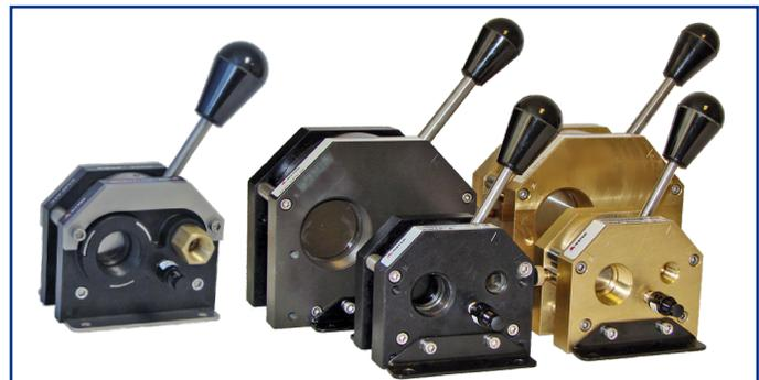
**3 FasTie Quick Ejector Tie-In** slashes knockout connection time to seconds with quick couplers and pull studs. FasTie couplers reside in the press ejector plate. FasTie pull studs are fastened to each mold in storage. When a mold change is performed, ejector tie in is literally a snap.
